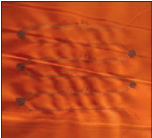
Fig. 3. F-TEG type T Pairs of legs of Constantan and Copper threads Junctions consolidated by Silver threads Electric circuit Ohmic resistance: 55 \Omega
